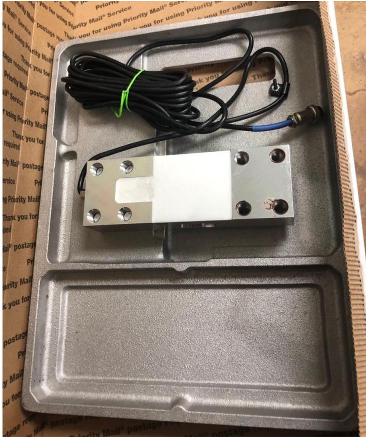
Remove the painted top, using an Allen wrench. Your scale may look like the attached photo. Remove the strain relief next to the carry handle. The wire does not unplug from the load cell. As you can see in photo it does unplug from the indicator end. Notice this photo shows the color code BLUE.
